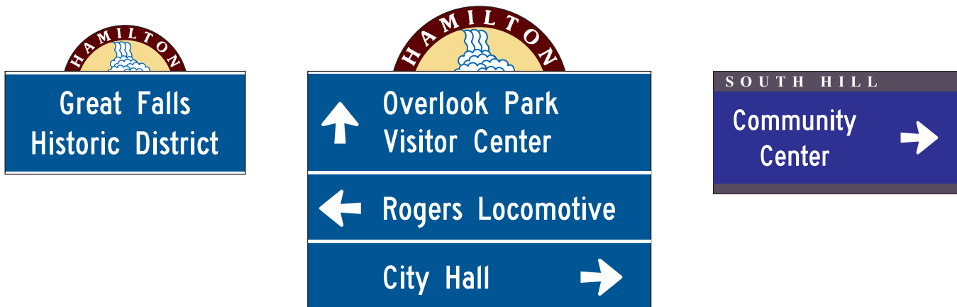
Figure 2D-18. Examples of Community Wayfinding Guide Signs
