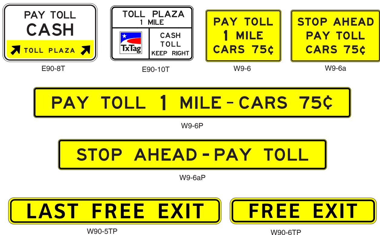
Figure 2F-3. Toll Plaza Warning Signs and Plaques
