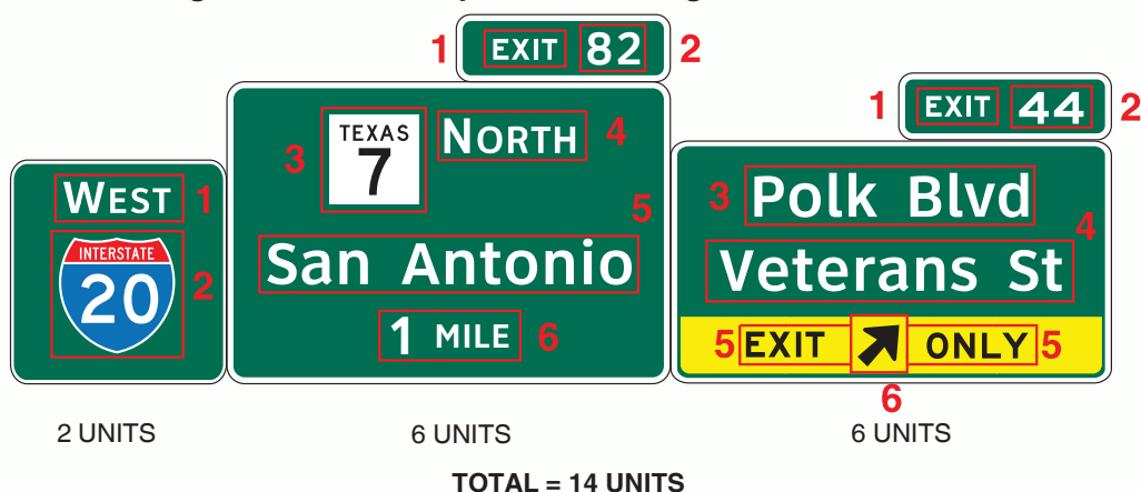
Figure 2E-1T Example of Guide Sign Information Units
